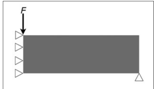
Figure 3. Half MBB structure: the lower right most atom is fixed vertically, while all atoms on the leftmost column are fixed horizontally. A downward force of 1 Newton is applied to the top rightmost atom. The design space is 150x50 atoms. The volume fraction of material (i.e. the initial density of each element) is 0.5.
