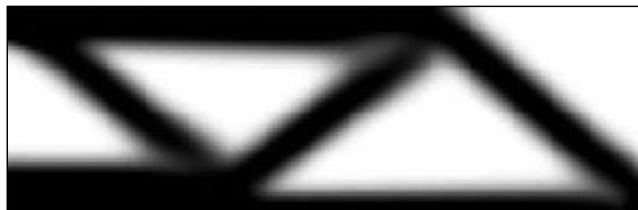
Figure 4. FE configuration. Compliance = 27.7525 \text{ Pa}^{-1} .
